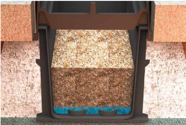
Water reservoir in the lower section
