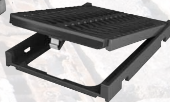
Cast-iron cover Cl. A/B 125 kN, incl. cast-iron frame and connection clamps made of spring steel incl. child safeguard
